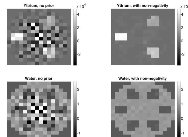
smeared by Gaussian noise with **5 different metallic filters**  $F_i$ , which are ideal pass-band filters around the discontinuities specifying the contrast agents. The discretized sizes are  $M = 1440$ ,  $D = 256$ , and  $N = 43$ .
